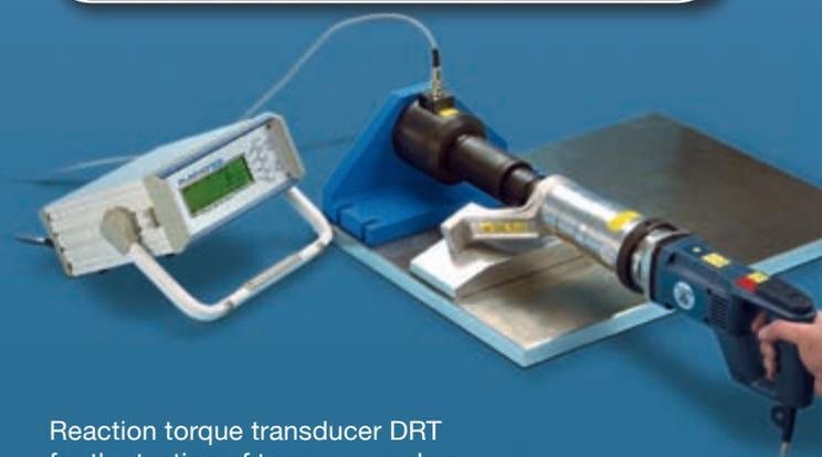
Reaction torque transducer DRT for the testing of torque wrenches, electrical and pneumatic torque wrenches and impact tools of various types.
