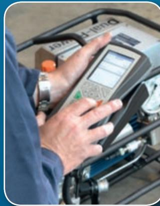
Operation of the power pack takes place by means of a user-friendly remote control unit. The remote control unit for the IQ power packs has a display indicating the parameters voltage, current, temperature, pressure, torque and rotation angle (in the case of rotation angle technique).
