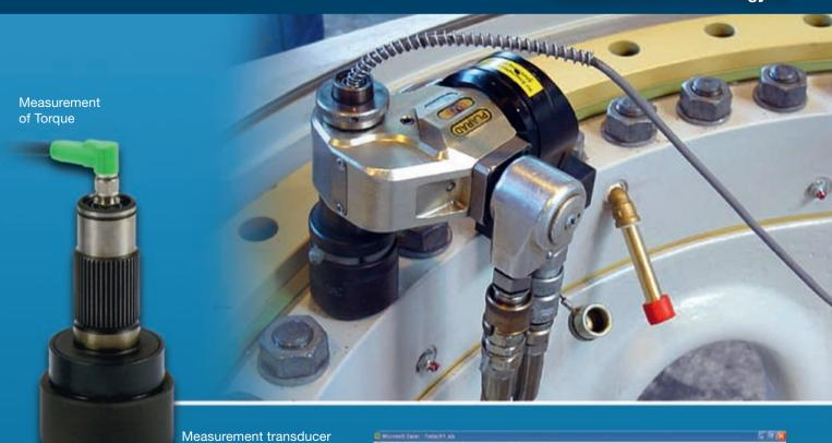
The measured values are saved with the date and time and can be printed out directly from the unit or transferred to a PC for
