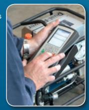
Operation of the power pack takes place by means of a user-friendly remote control unit. The remote control unit for the IQ power packs has a display indicating the parameters voltage, current, temperature, pressure, torque and rotation angle (in the case of rotation angle technique).
